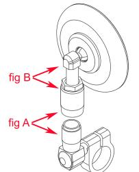
STEP 5: Once desired mirror length and angle is determined use a 12mm wrench to hold rod head (fig B) while tightening 16mm nut. Tighten clamp bolt (fig C). Check there is no interference before riding with throttle, brake, clutch and any other parts.
