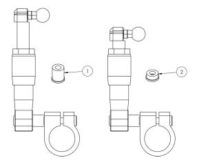
STEP 2: Install in the sequence illustrated below using the flathead bolt. Apply blue thread locking agent.
